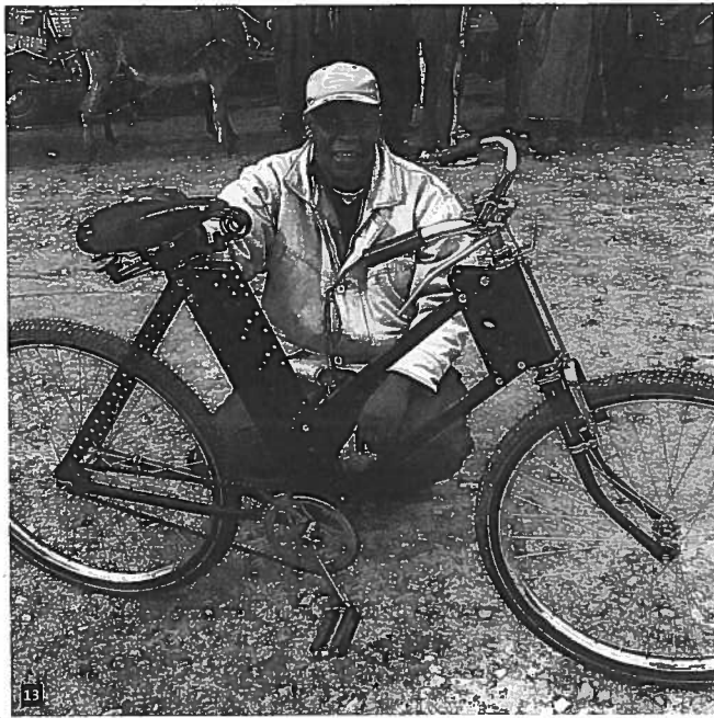
13. A bicycle fabricated using the Design With Africa bicycle modules, Rustenburg, South Africa.
